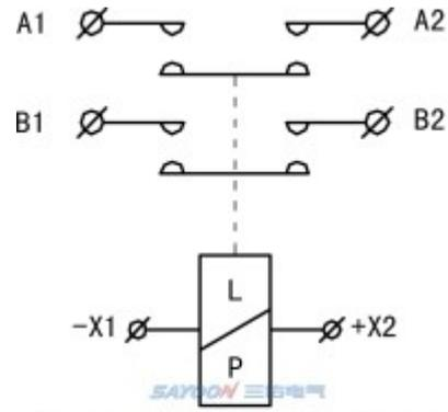
AH Double Pole Double Throw Contactor. (Two Normally Open)
