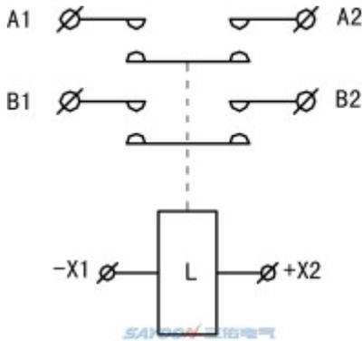
AD Double Pole Double Throw Contactor. (Two Normally Open)
