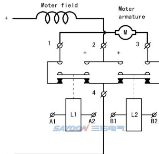
Paired Single Pole Double Throw Contactor for motor reversing
